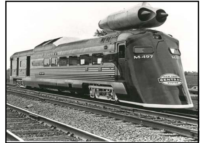
In 1966, this jet-powered railcar set the North American rail speed record through Stryker
